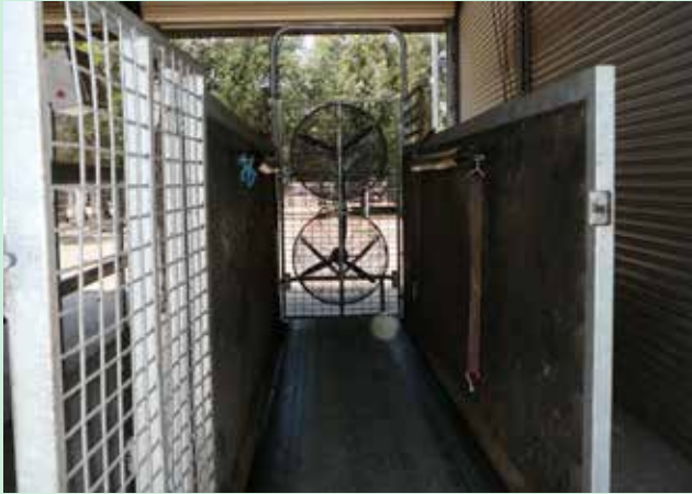
A horse treadmill with caged fans
