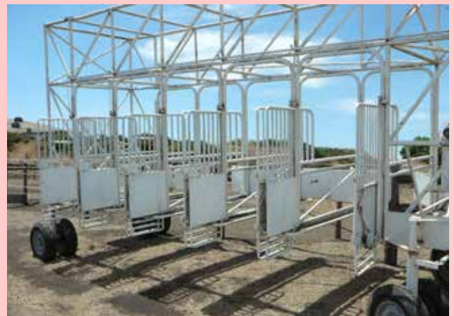
No padding or protection on gates/barriers
