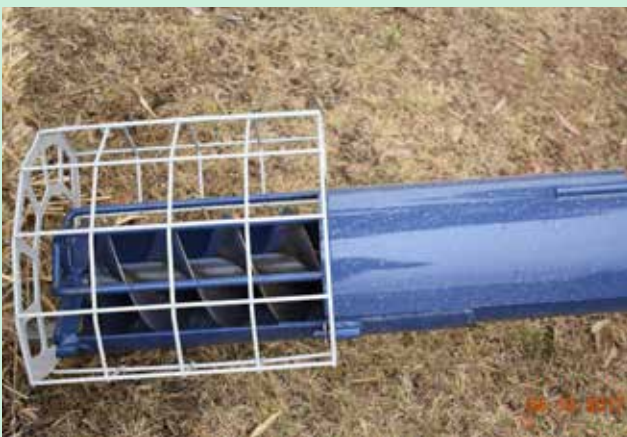
Appropriate guarding on an auger
