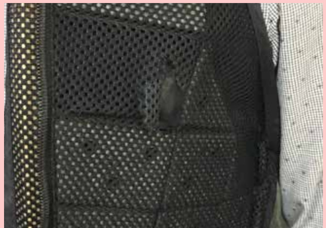
Vest damaged and torn as impact panel has been removed
