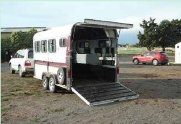
This vehicle is designed to allow improved safe loading, unloading and maintenance of horses without being exposed to significant entrapment or crushing hazards by the horse - safe access to the entire length of a horse is possible with this design
